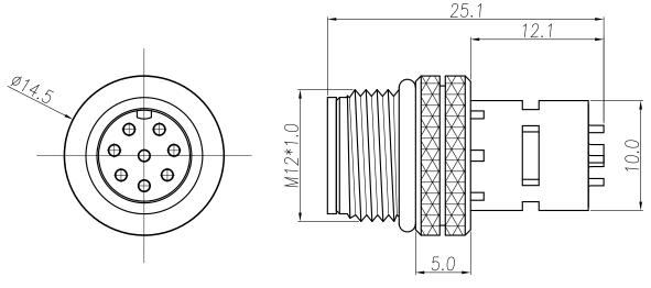
NOTE: MATERIAL HDUSING: PBT UL94V-0, BLACK CONTACT: BRASS SHELL: BRASS NUT: BRASS EPDM, BLACK □-RING: FINISH CONTACT: GOLD PLATED □VER 504" NICKEL SHELL: BRIGHT TIN NUT: NICKEL PLATED **ELECTRICAL** RATED CURRENT: 2A RATED VOLTAGE: 30V 100 MOhms MIN. INSULATION RESISTANCE: 10 mOhms MAX. CONTACT RESISTANCE: WATER PROOF: IP67 **ENVIRONMENT** OPERATION TEMPERATURE: -40°C TD +85°C MAX WIRE AWG: 24
