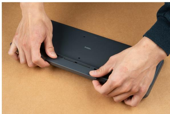
Flipping over the cover, you'll notice that the dongle is attached inconspicuously on the back. Grab the wireless dongle from the back to insert into the Pi's USB port and slide the cover back on the Logitech K400 Plus.
