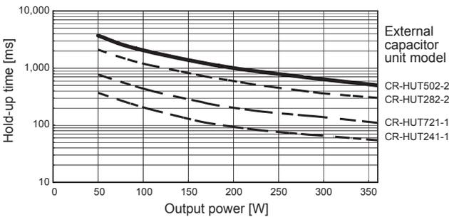
Fig.7.6 Hold-up time by LFP300F-TU1Y(Reference data).
