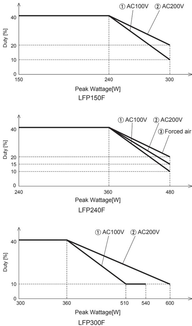
Fig.6.1 Derating of peak loading
