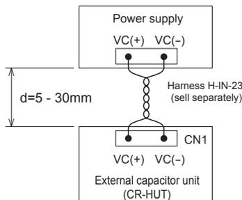
Fig.7.7 Connection method
