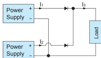
Fig.2.2 Example of redundancy operation
