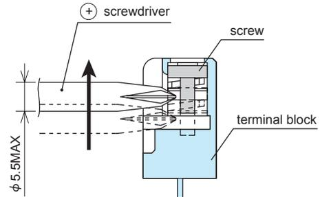
Fig.7.3 lifting method
