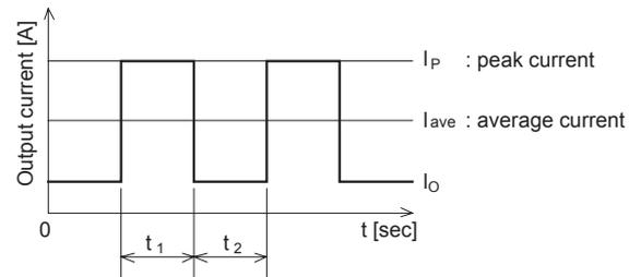
$$t_1 \leq 10 \text{ [sec]}, I_{ave} = \frac{I_p \cdot t_1 + I_o \cdot t_2}{t_1 + t_2} \leq \text{rated current,}$$
