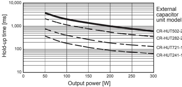
Fig.7.5 Hold-up time by LFP240F-U1Y(Reference data).
