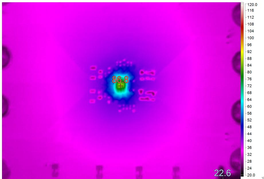
Figure 2. Thermal Image with 3.1V<sub>IN1</sub>, 3.1V<sub>IN2</sub>, 2.5V<sub>OUT1</sub> at 2.5A and 2.5V<sub>OUT2</sub> at 2.5A. Vertical Orientation with No Forced Air.
