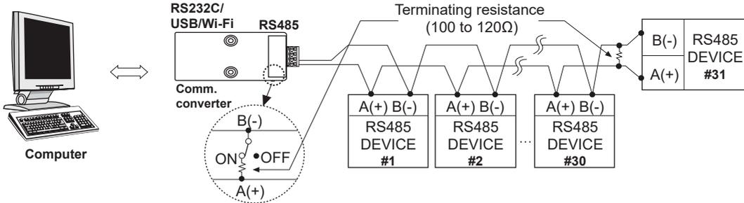
※It is recommended to use Autonics communication converter; SCM-WF48 (Wi-Fi to RS485-USB wireless communication converter, sold separately), SCM-US48I (USB to RS485 converter, sold separately), SCM-38I (RS232C to RS485 converter, sold separately).
