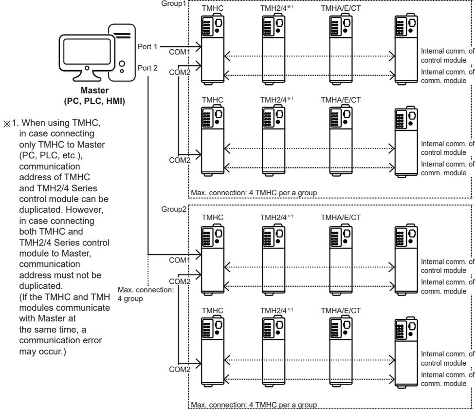
⊗ 1. When using TMHC, in case connecting only TMHC to Master (PC, PLC, etc.), communication address of TMHC and TMH2/4 Series control module can be duplicated. However, in case connecting both TMHC and TMH2/4 Series control module to Master, communication address must not be duplicated. (If the TMHC and TMH modules communicate with Master at the same time, a communication error may occur.)
