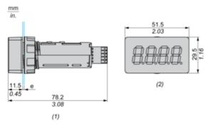
e: Clamping thickness 1 to 6 mm
