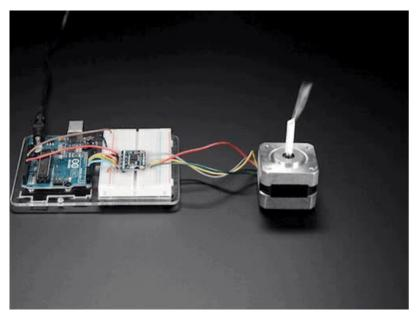
We solder on TB6612 onto a breakout board for you here, with a polarity protection FET on the motor voltage input and a pullup on the "standby" enable pin. Each breakout chip contains two full H-bridges (four half H-bridges). That means you can drive four solenoids, two DC motors bi-directionally, or one stepper motor. Just make sure they're good for 1.2 Amp or less of current, since that's the limit of this chip.
