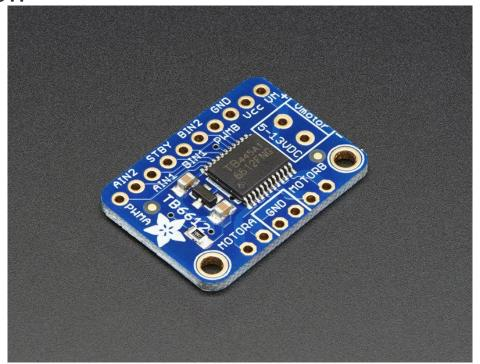
Fire four solenoids, spin two DC motors or step one bi-polar or uni-polar stepper with 1.2A per channel using the TB6612. These are perhaps better known as "the drivers in our assembled Adafruit Motorshield (http://adafru.it/1438) or Motor HAT (https://adafru.it/eRq)" We really like these dual H-bridges, so if you want to control motors without a shield or HAT these are easy to include on any solderless breadboard or perma-proto.
