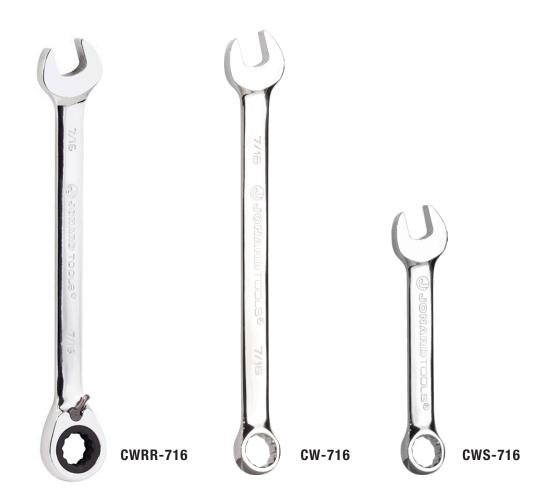
Measures 7/16" at both the open end and box end. Both ends have an angle offset (15°) to ease access in confined areas. The box end offers 12 points of contact. Chrome plated, polished to a high gloss finish and made of chrome vanadium steel.
