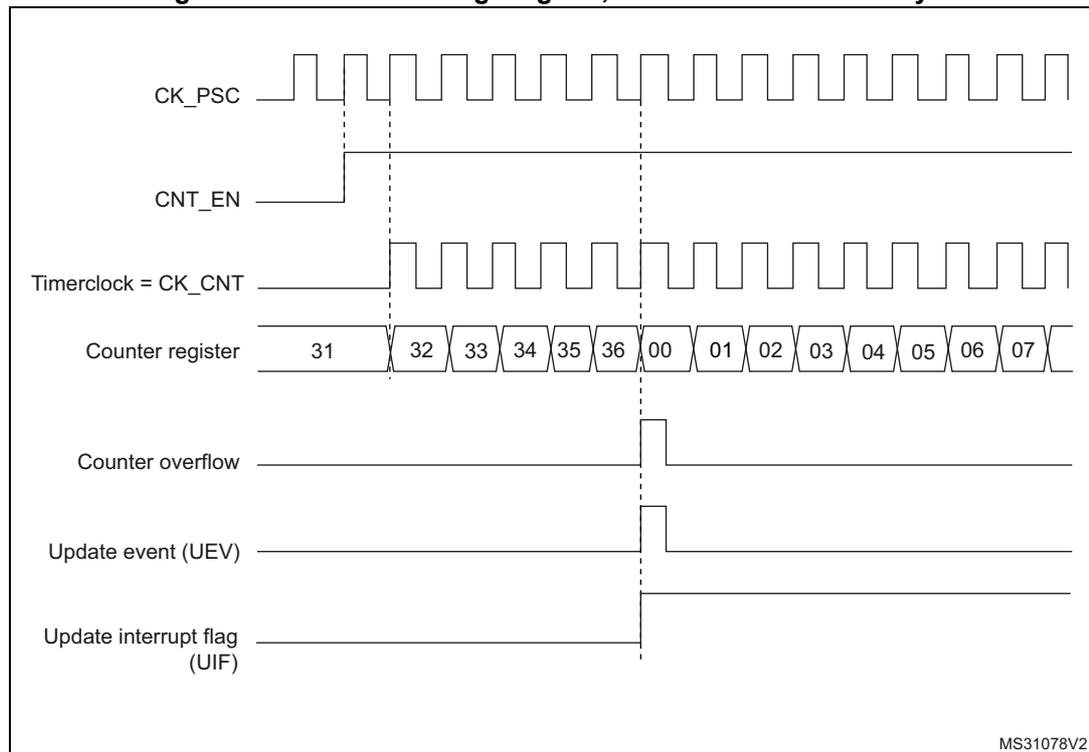
Figure 205. Counter timing diagram, internal clock divided by 2
