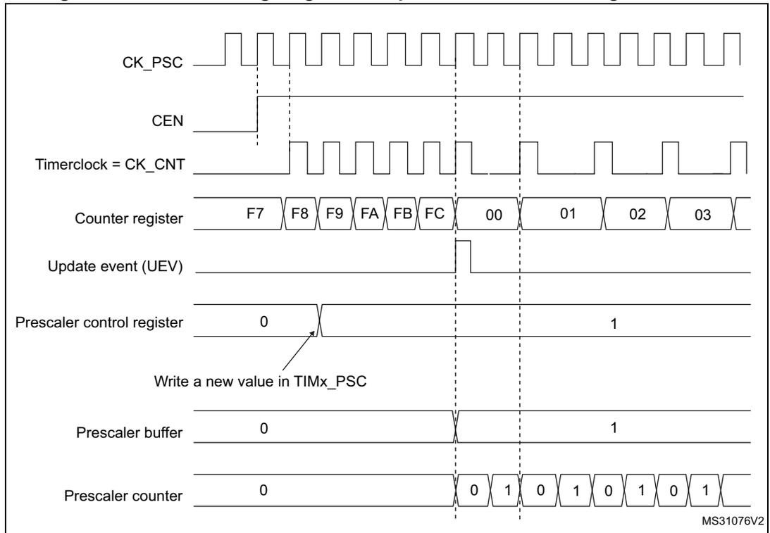
Figure 65. Counter timing diagram with prescaler division change from 1 to 4
