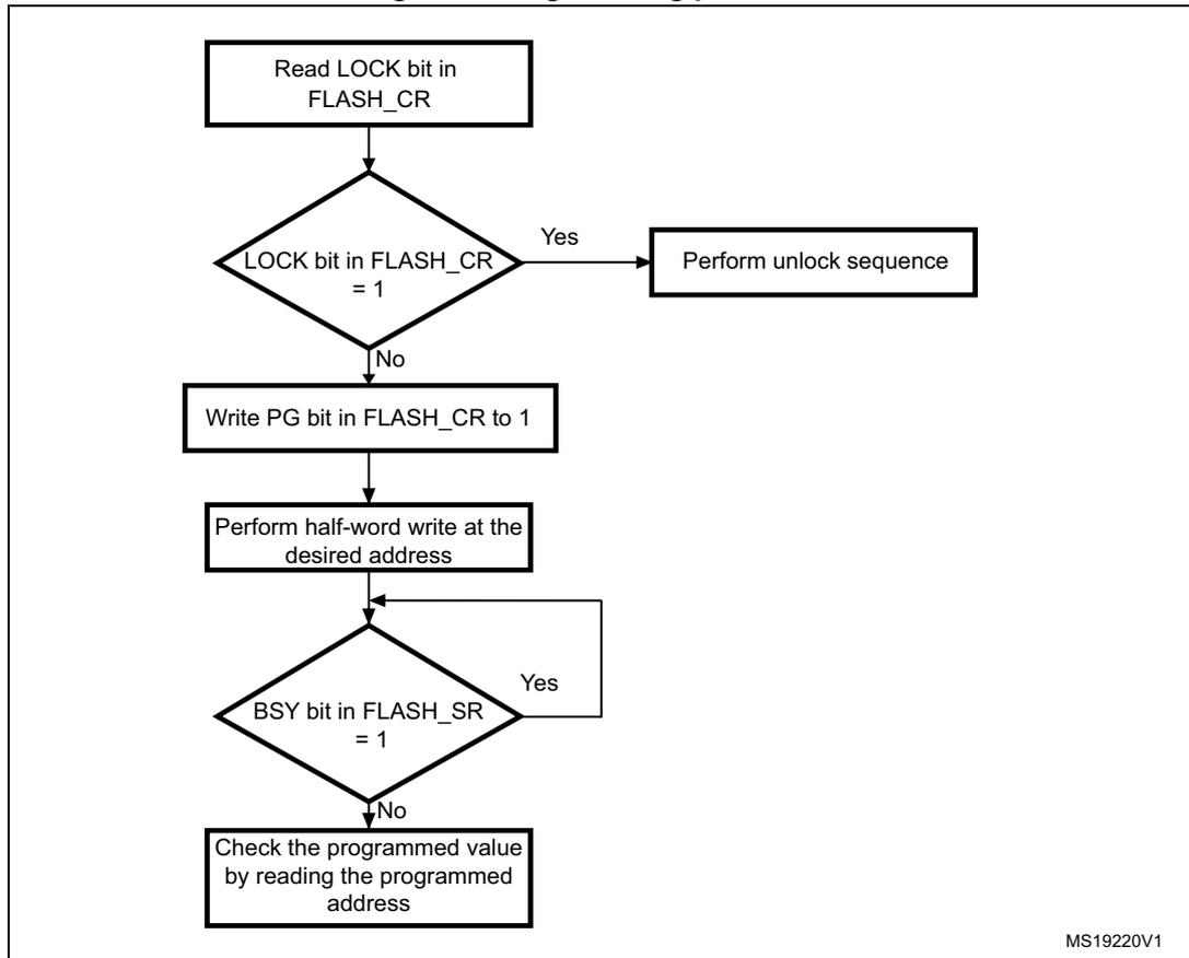
The flash memory interface preliminarily reads the value at the addressed main flash memory location and checks that it has been erased. If not, the program operation is skipped and a warning is issued by the PGERR bit in FLASH\_SR register. The only exception to this is when 0x0000 is programmed. In this case, the location is correctly programmed to 0x0000 and the PGERR bit is not set.
