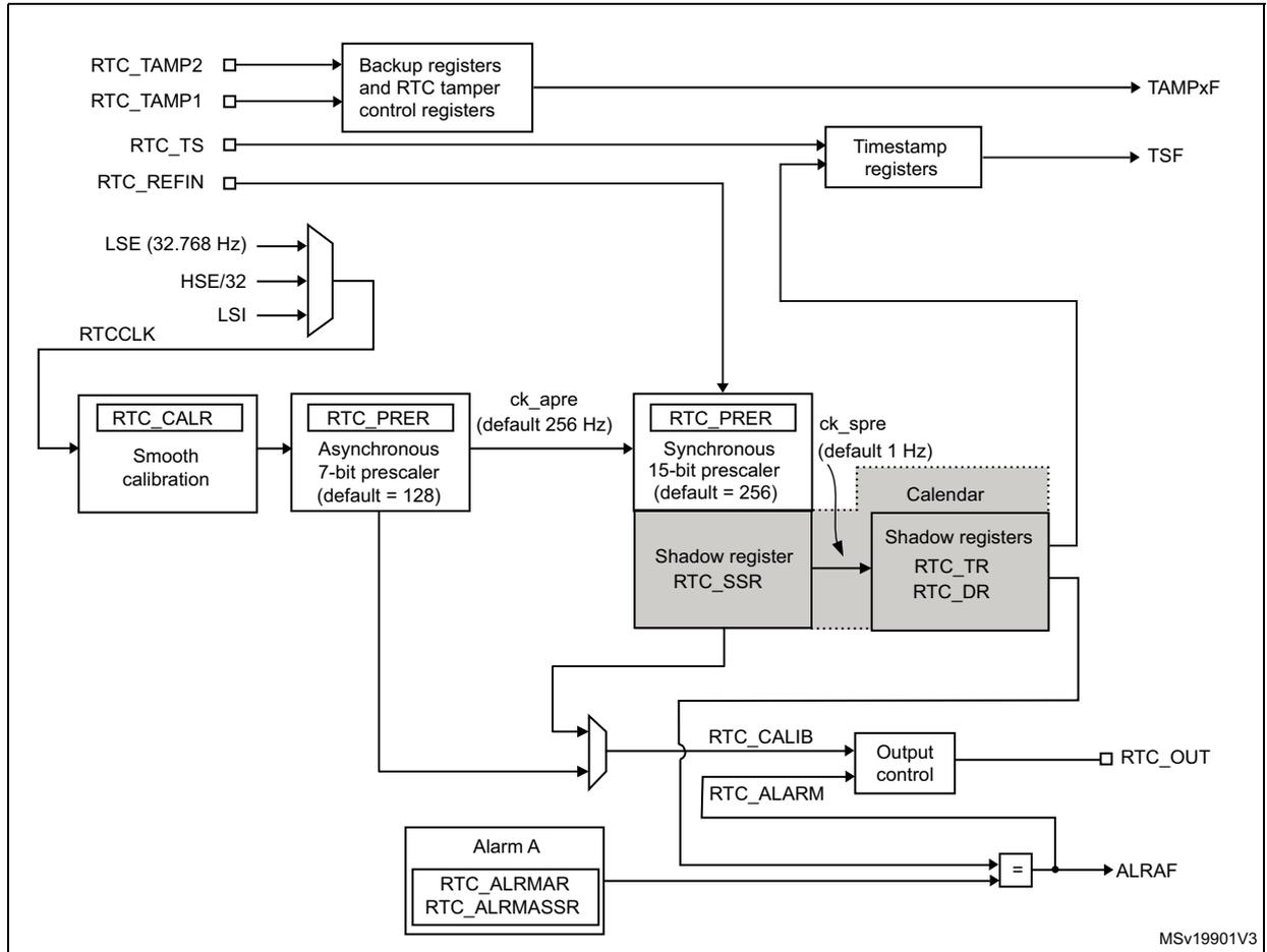
Figure 216. RTC block diagram for STM32F07x and STM32F09x devices
