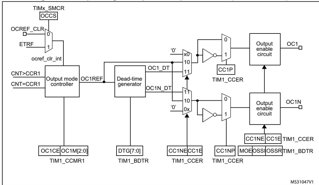
Figure 92. Output stage of capture/compare channel (channel 4)
