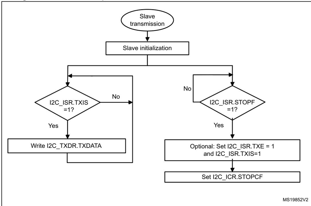
**Figure 227. Transfer bus diagrams for I2C slave transmitter (mandatory events only)**
