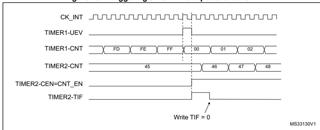
As in the previous example, both counters can be initialized before starting counting. [Figure 155](#) shows the behavior with the same configuration as in [Figure 154](#) but in trigger mode instead of gated mode (SMS=110 in the TIM2\_SMCR register).
