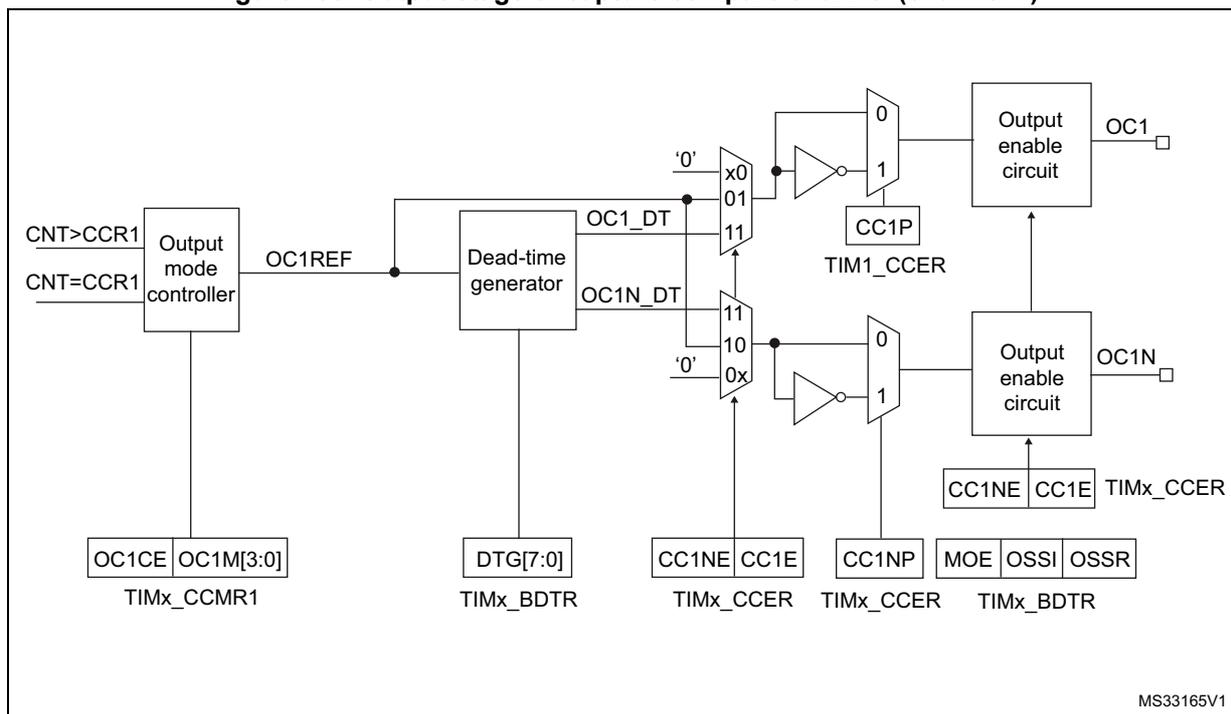
Figure 189. Output stage of capture/compare channel (channel 2 for TIM15)
