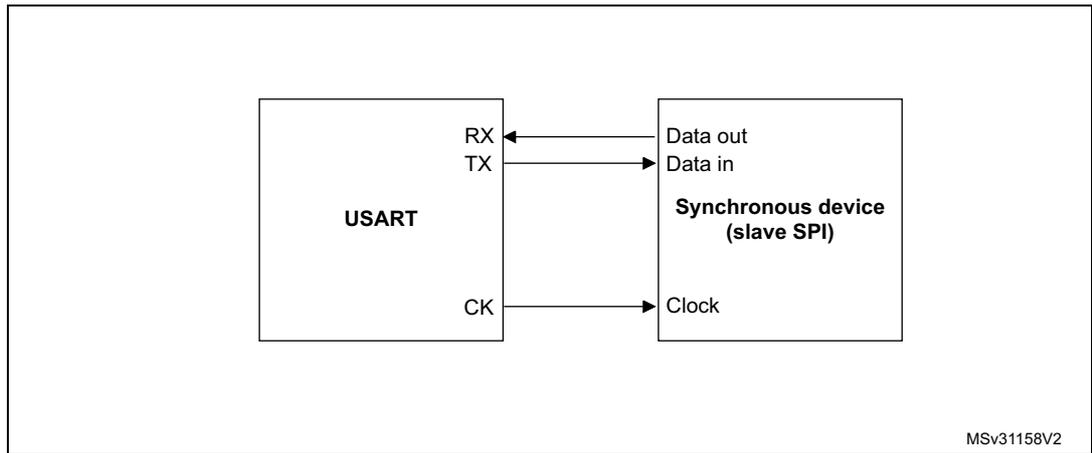
**Figure 260. USART data clock timing diagram (M bits = 00)**
