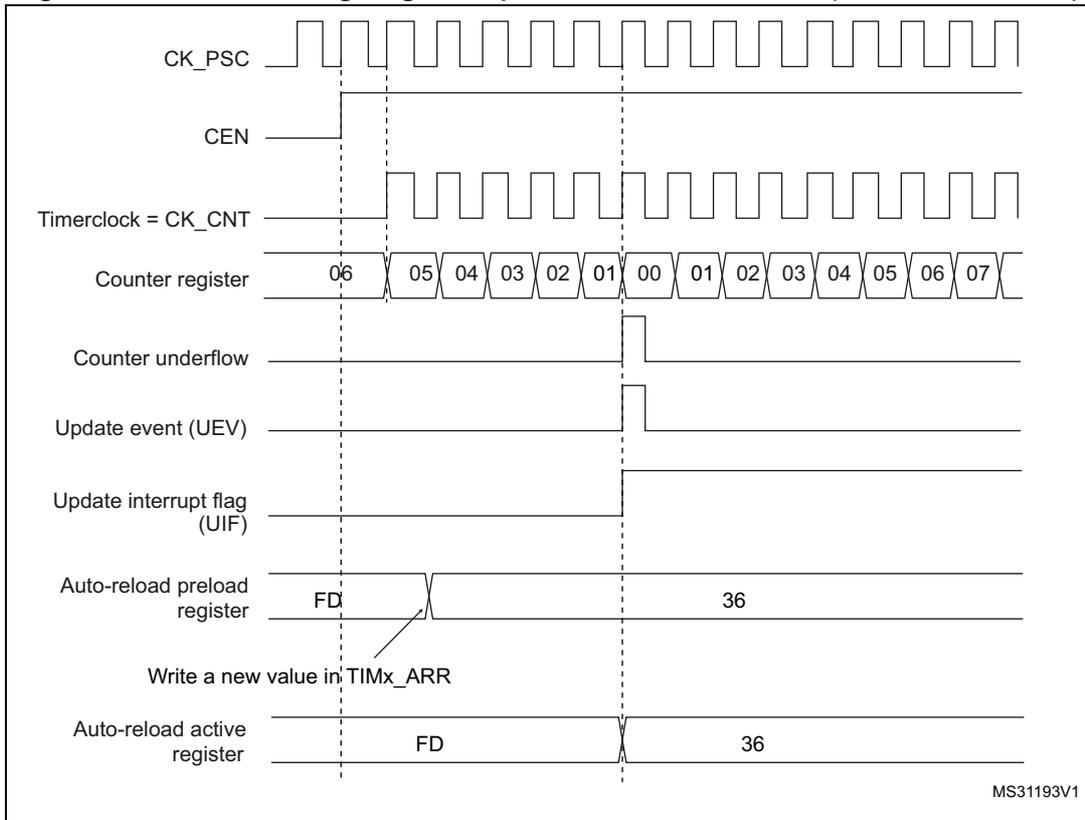
Figure 130. Counter timing diagram, Update event with ARPE=1 (counter overflow)
