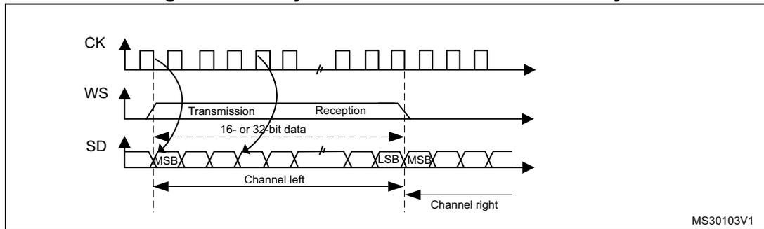
**Figure 301. LSB justified 24-bit frame length**
