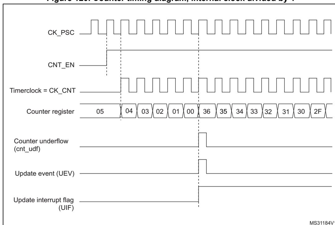
**Figure 121. Counter timing diagram, internal clock divided by 2**
