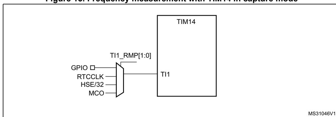
The input capture channel of the Timer 14 can be a GPIO line or an internal clock of the MCU. This selection is performed through the TI1\_RMP [1:0] bits in the TIM14\_OR register. The possibilities available are the following ones.
