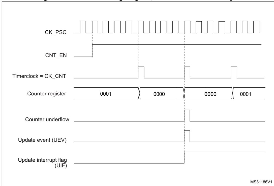
Figure 123. Counter timing diagram, internal clock divided by N
