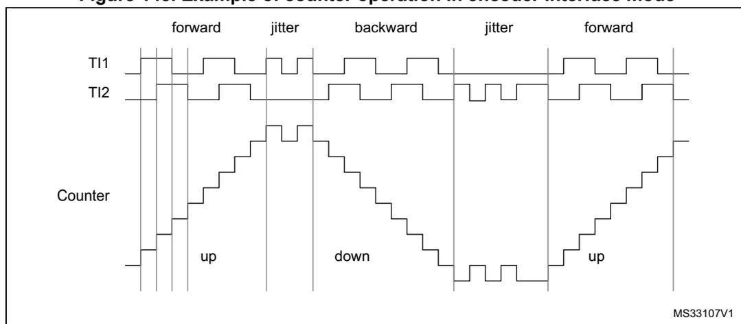
Figure 146 gives an example of counter behavior when TI1FP1 polarity is inverted (same configuration as above except CC1P=1).
