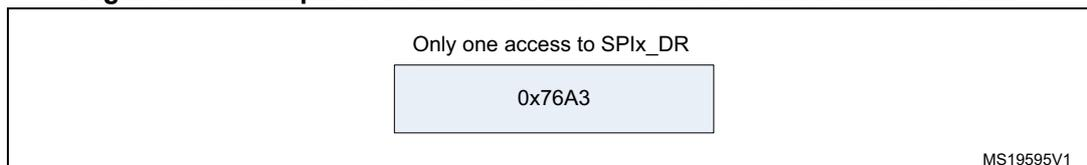
For transmission, each time an MSB is written to SPIx\_DR, the TXE flag is set and its interrupt, if allowed, is generated to load the SPIx\_DR register with the new value to send. This takes place even if 0x0000 have not yet been sent because it is done by hardware.
