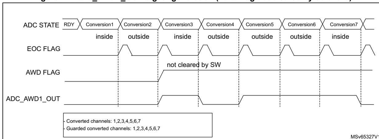
Figure 45. ADC1\_AWD\_OUT signal generation (on a single channel)
