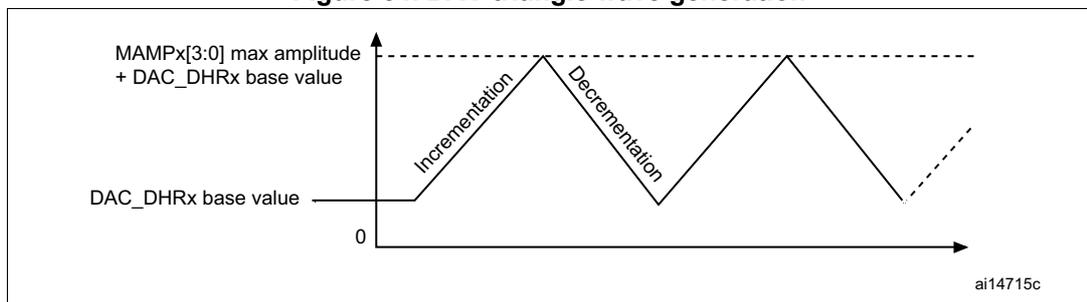
**Figure 55. DAC conversion (SW trigger enabled) with triangle wave generation**
