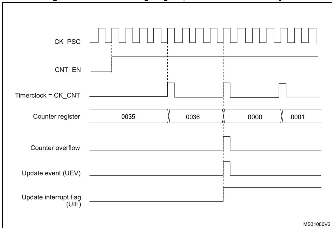
Figure 179. Counter timing diagram, internal clock divided by N
