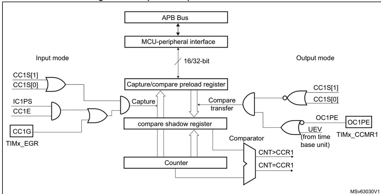
Figure 188. Output stage of capture/compare channel (channel 1)
