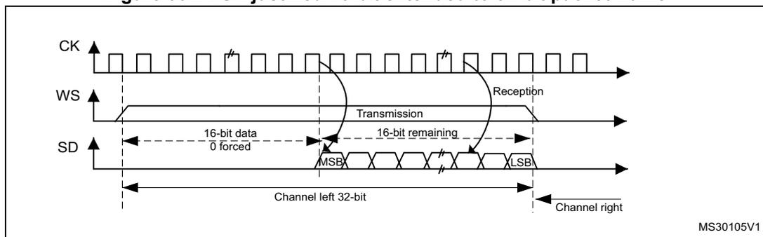
When 16-bit data frame extended to 32-bit channel frame is selected during the I2S configuration phase, Only one access to the SPIx\_DR register is required. The 16 remaining bits are forced by hardware to 0x0000 to extend the data to 32-bit format. In this case it corresponds to the half-word MSB.
