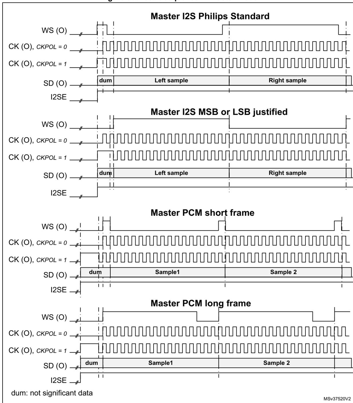
In slave mode, the user has to enable the audio interface before the WS becomes active. This means that the I2SE bit must be set to 1 when WS = 1 for I<sup>2</sup>S Philips standard, or when WS = 0 for other standards.
