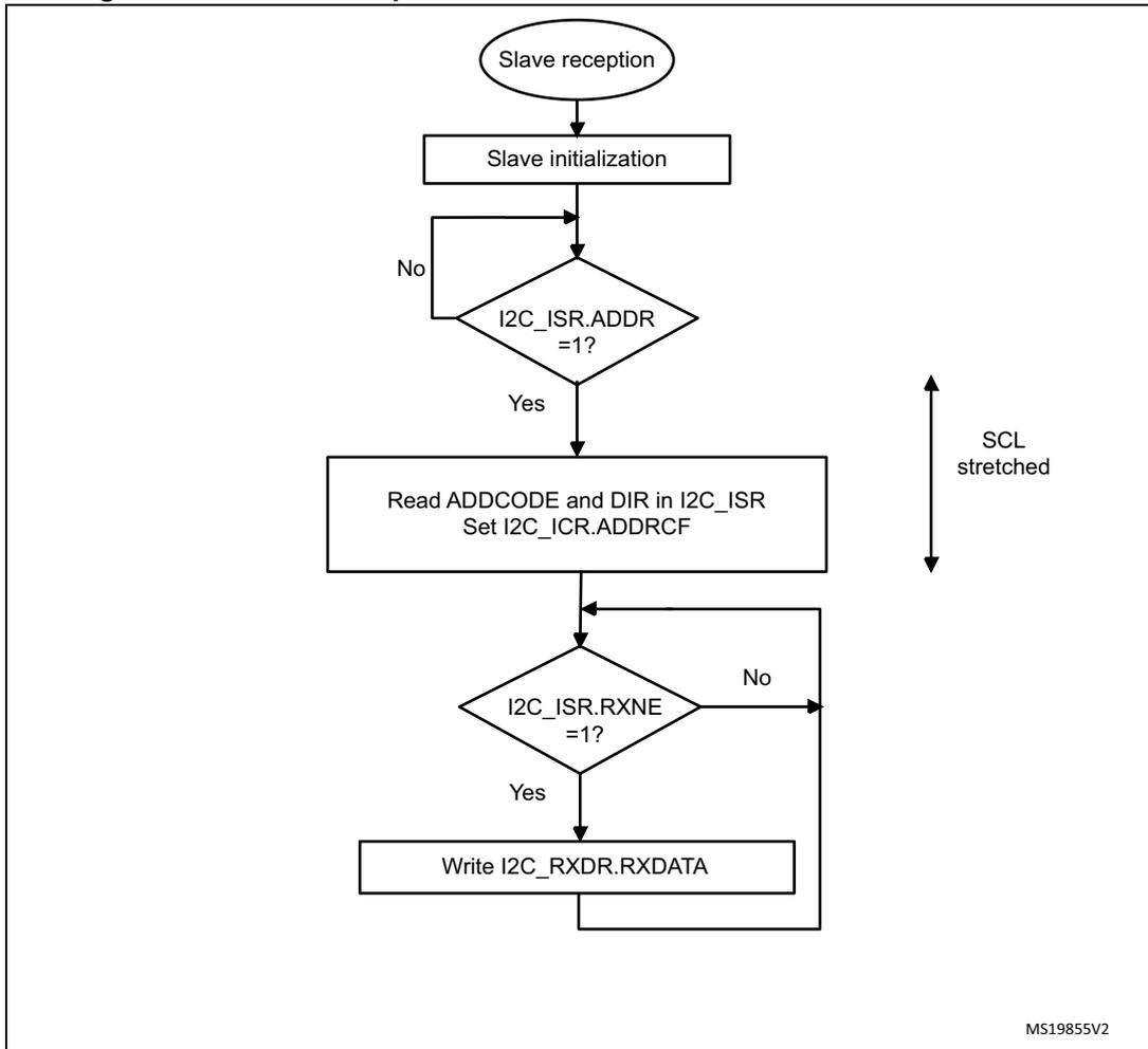
Figure 229. Transfer sequence flow for slave receiver with NOSTRETCH = 1
