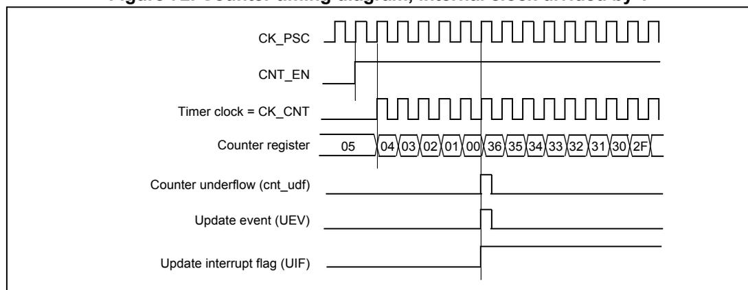
**Figure 73. Counter timing diagram, internal clock divided by 2**
