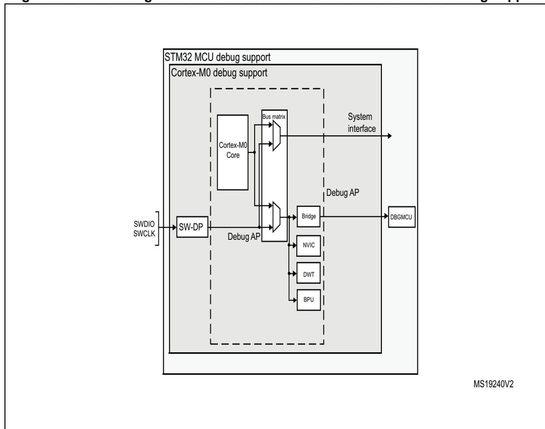
1. The debug features embedded in the Cortex<sup>®</sup>-M0 core are a subset of the Arm CoreSight Design Kit.
