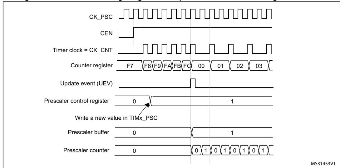
**Figure 159. Counter timing diagram with prescaler division change from 1 to 4**
