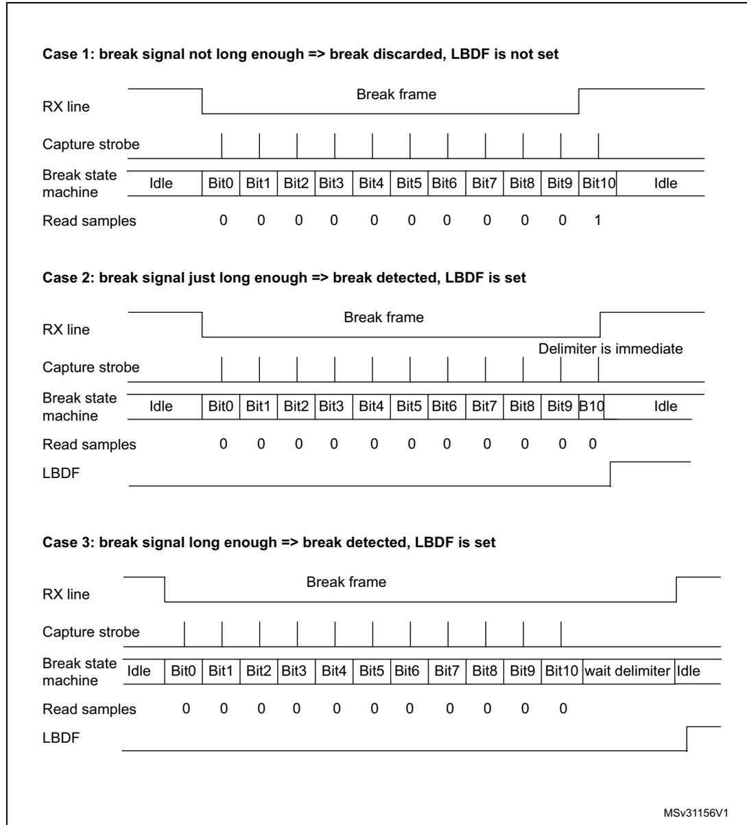
Figure 258. Break detection in LIN mode vs. Framing error detection
