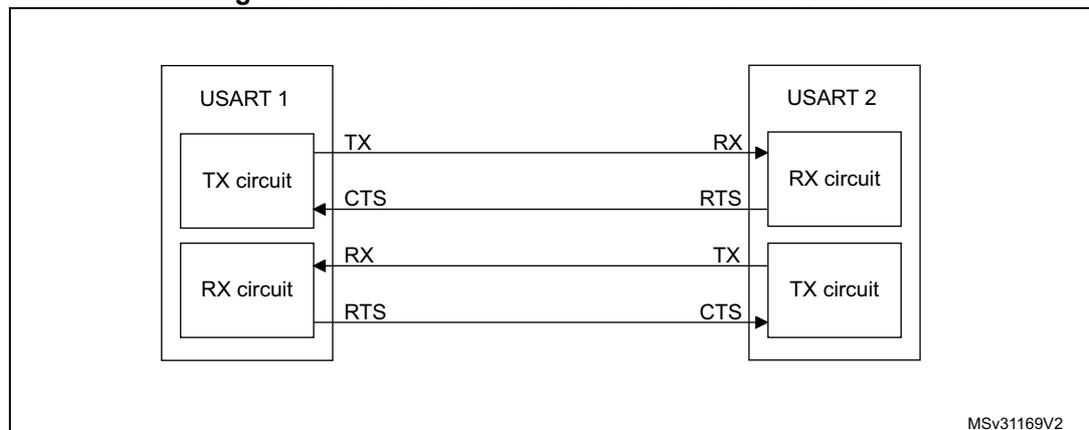
RS232 RTS and CTS flow control can be enabled independently by writing the RTSE and CTSE bits respectively to 1 (in the USART\_CR3 register).
