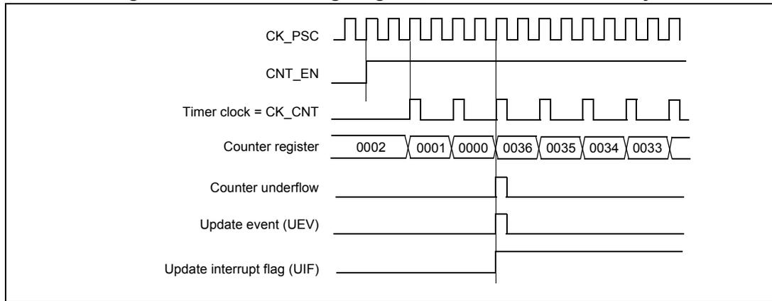
**Figure 74. Counter timing diagram, internal clock divided by 4**
