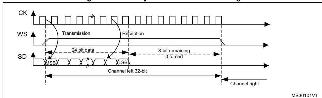
**Figure 299. MSB justified 16-bit extended to 32-bit packet frame**
