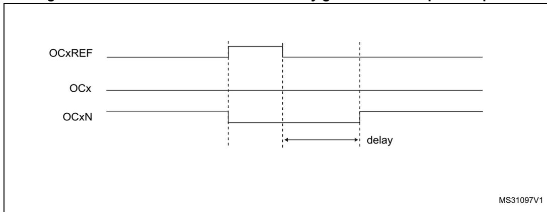
The dead-time delay is the same for each of the channels and is programmable with the DTG bits in the TIMx\_BDTR register. Refer to [Section 20.5.16: TIM15 break and dead-time register \(TIM15\\_BDTR\) on page 538](#) for delay calculation.
