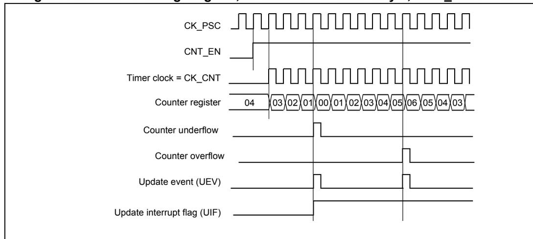
1. Here, center-aligned mode 1 is used (for more details refer to [Section 17.4: TIM1 registers on page 375](#)).
