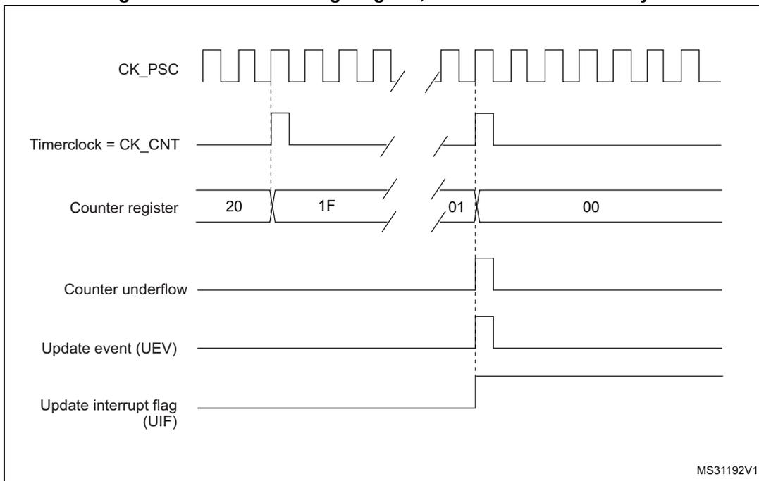
Figure 129. Counter timing diagram, Update event with ARPE=1 (counter underflow)
