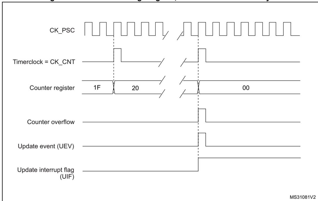
**Figure 118. Counter timing diagram, Update event when ARPE=0 (TIMx\_ARR not preloaded)**
