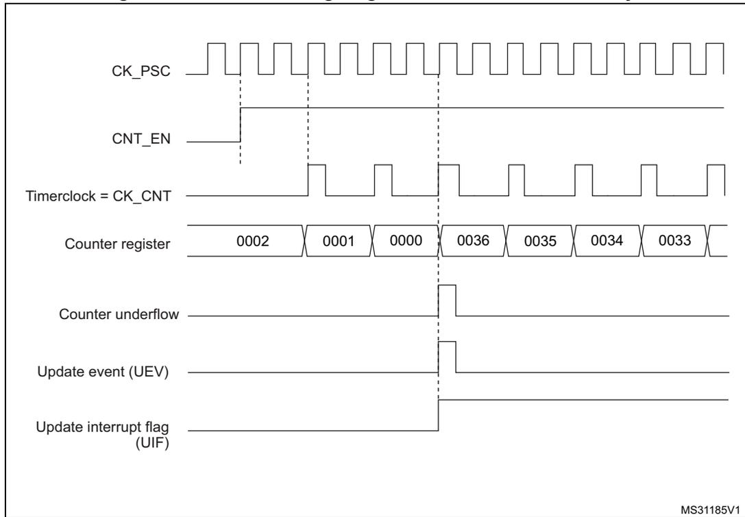
**Figure 122. Counter timing diagram, internal clock divided by 4**
