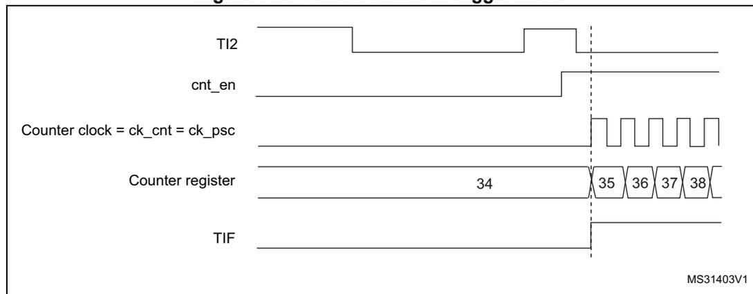
**Slave mode: External Clock mode 2 + trigger mode**
