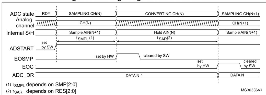
Figure 31. ADC conversion timings
