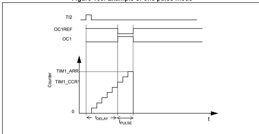
For example one may want to generate a positive pulse on OC1 with a length of t<sub>PULSE</sub> and after a delay of t<sub>DELAY</sub> as soon as a positive edge is detected on the TI2 input pin.
