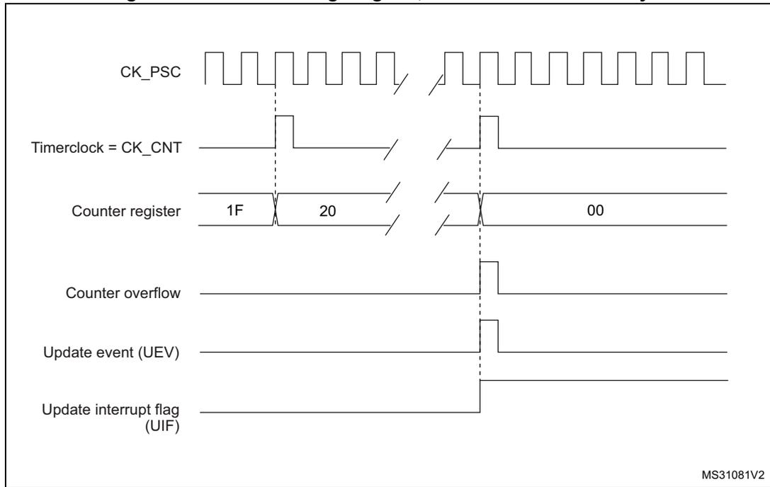
**Figure 70. Counter timing diagram, update event when ARPE=0 (TIMx\_ARR not preloaded)**
