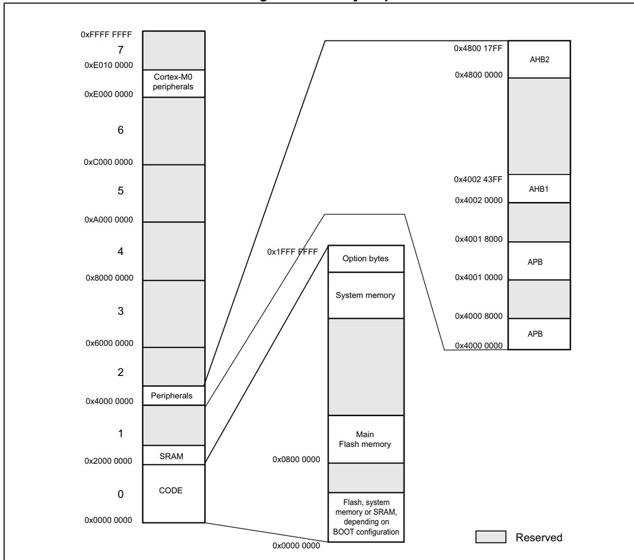
All the memory map areas not allocated to on-chip memories and peripherals are considered “Reserved”. For the detailed mapping of available memory and register areas, refer to the following table, which gives the boundary addresses of the available peripherals.
