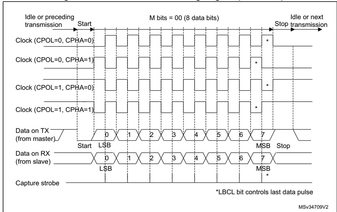
Figure 261. USART data clock timing diagram (M bits = 01)
