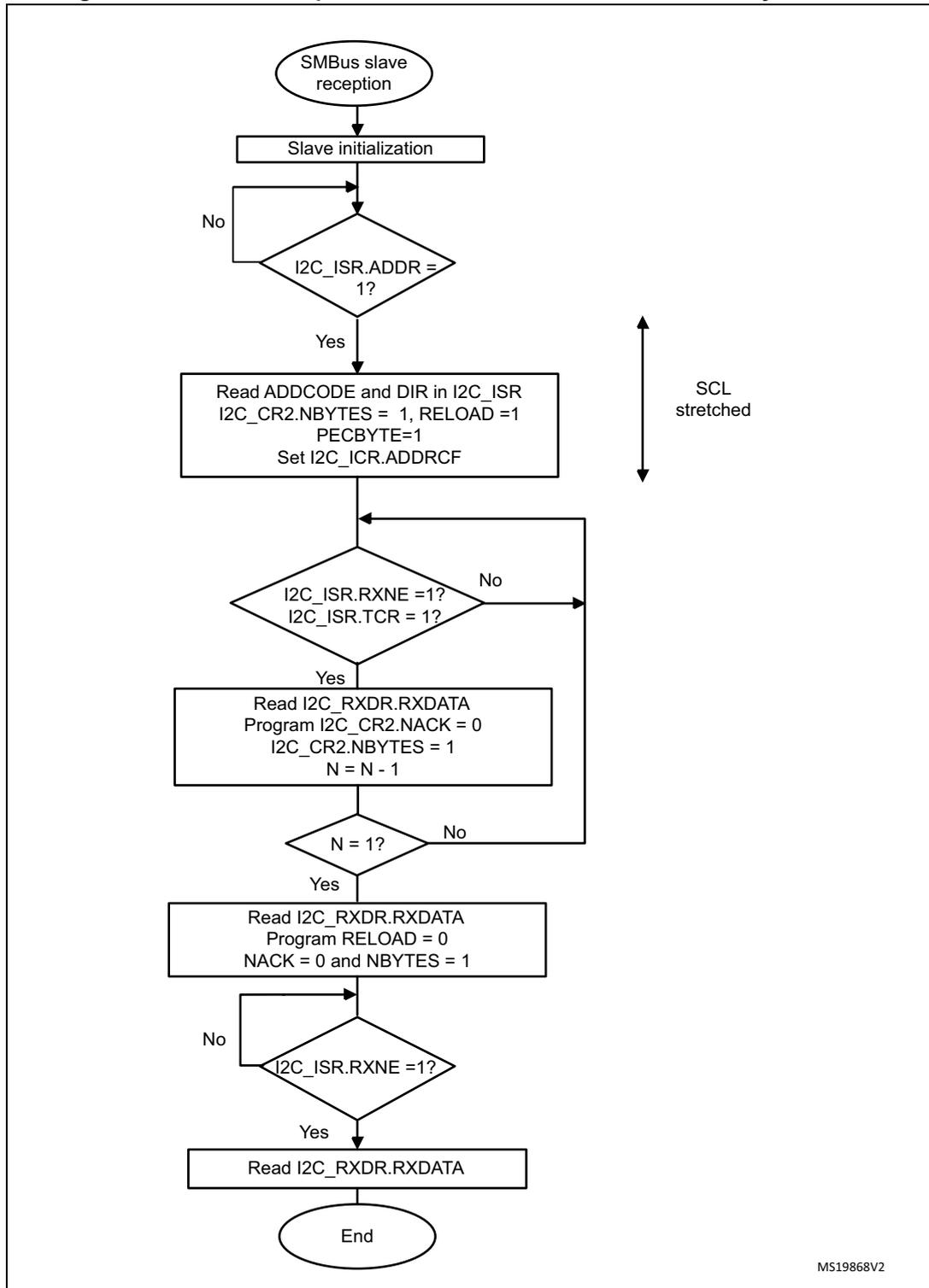
**Figure 245. Bus transfer diagrams for SMBus slave receiver (SBC = 1)**
