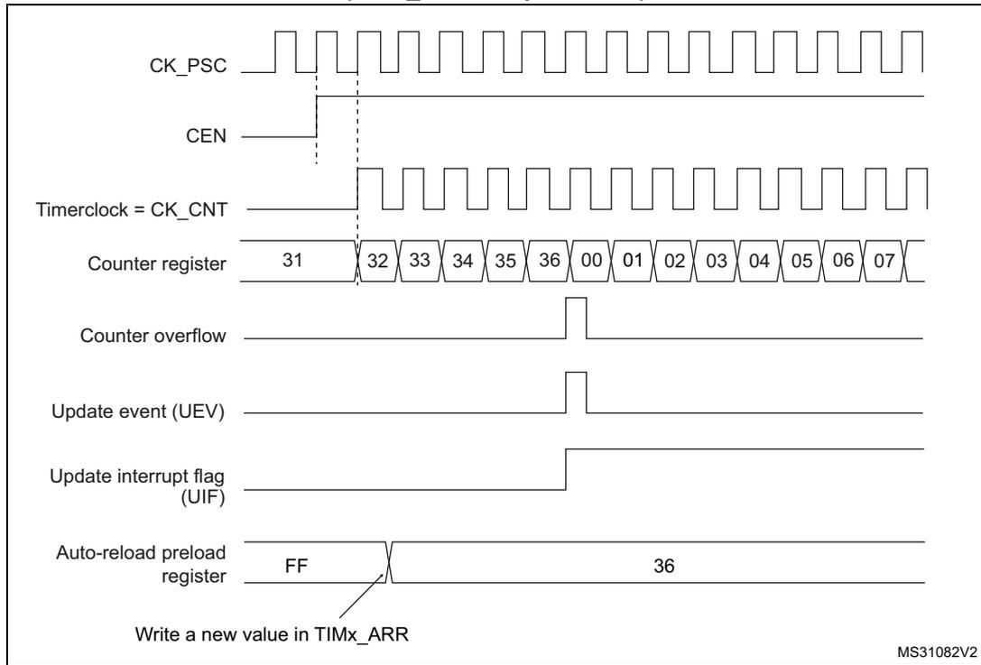
**Figure 119. Counter timing diagram, Update event when ARPE=1 (TIMx\_ARR preloaded)**
