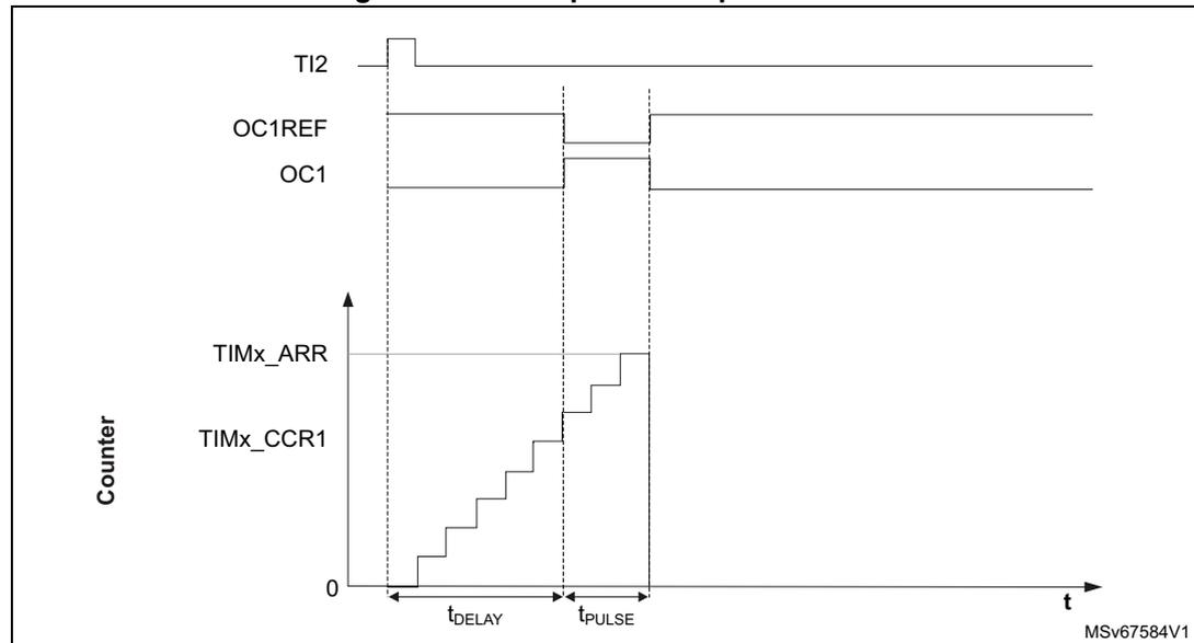
For example one may want to generate a positive pulse on OC1 with a length of  $t_{PULSE}$  and after a delay of  $t_{DELAY}$  as soon as a positive edge is detected on the TI2 input pin.
