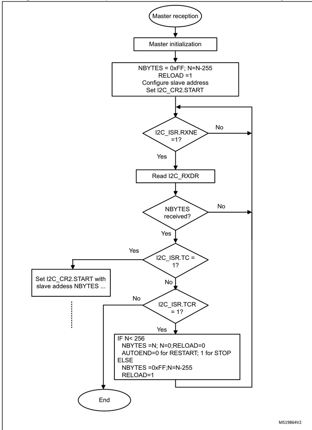
**Figure 240. Transfer bus diagrams for I2C master receiver (mandatory events only)**
