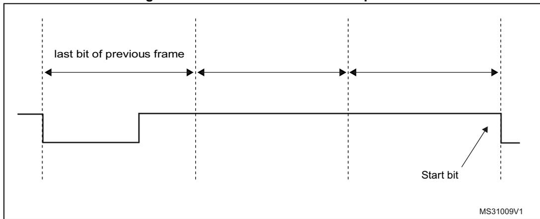
A configurable time window is counted before starting the transmission.
