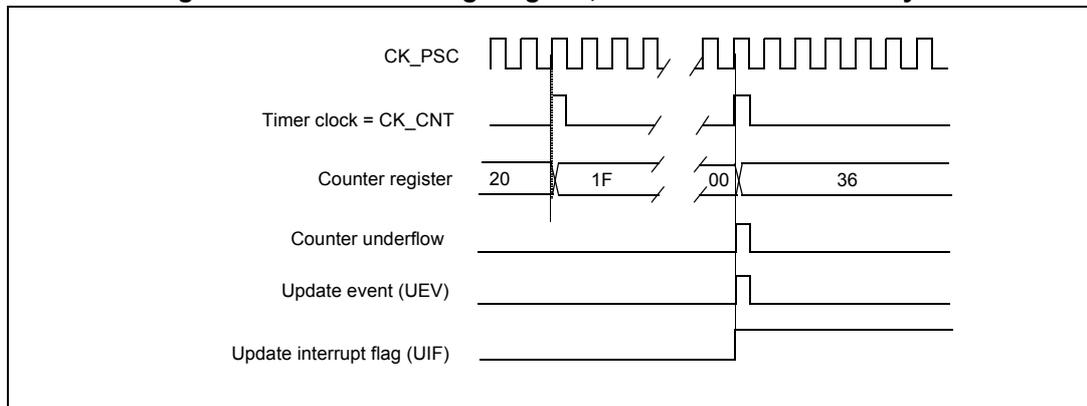
**Figure 76. Counter timing diagram, update event when repetition counter is not used**
