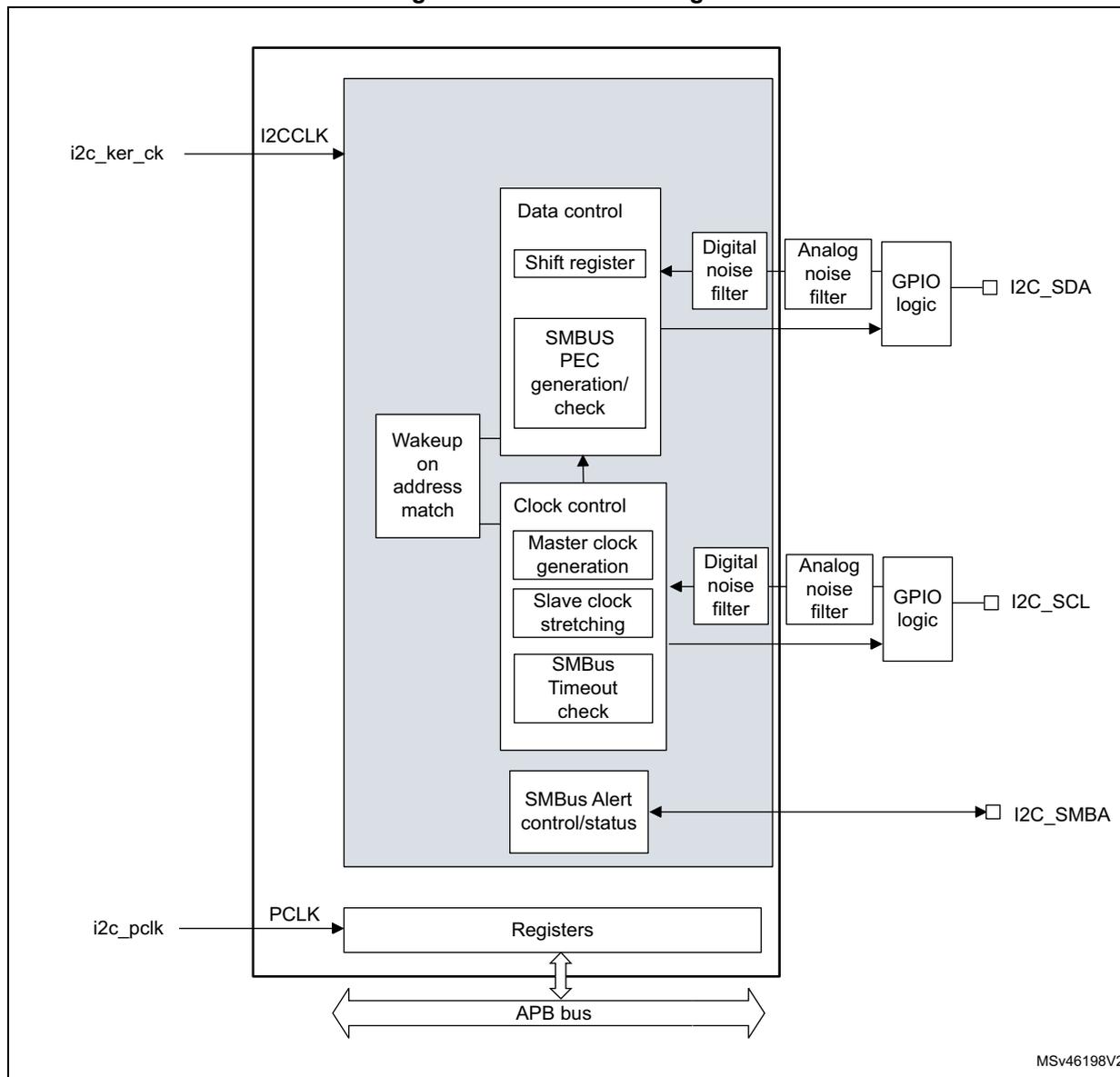
The I2C1 is clocked by an independent clock source, which allows the I2C to operate independently from the PCLK frequency.
