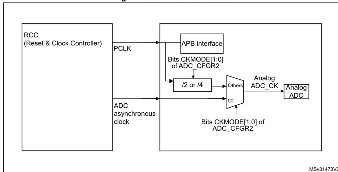
1. Refer to *Section Reset and clock control (RCC)* for how the PCLK clock and ADC asynchronous clock are enabled.
