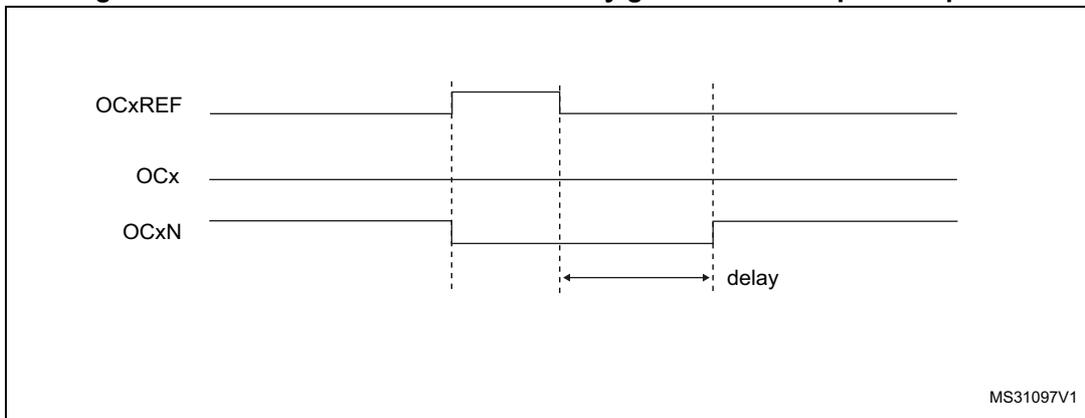
The dead-time delay is the same for each of the channels and is programmable with the DTG bits in the TIMx\_BDTR register. Refer to [Section 17.4.18: TIM1 break and dead-time register \(TIM1\\_BDTR\) on page 398](#) for delay calculation.
