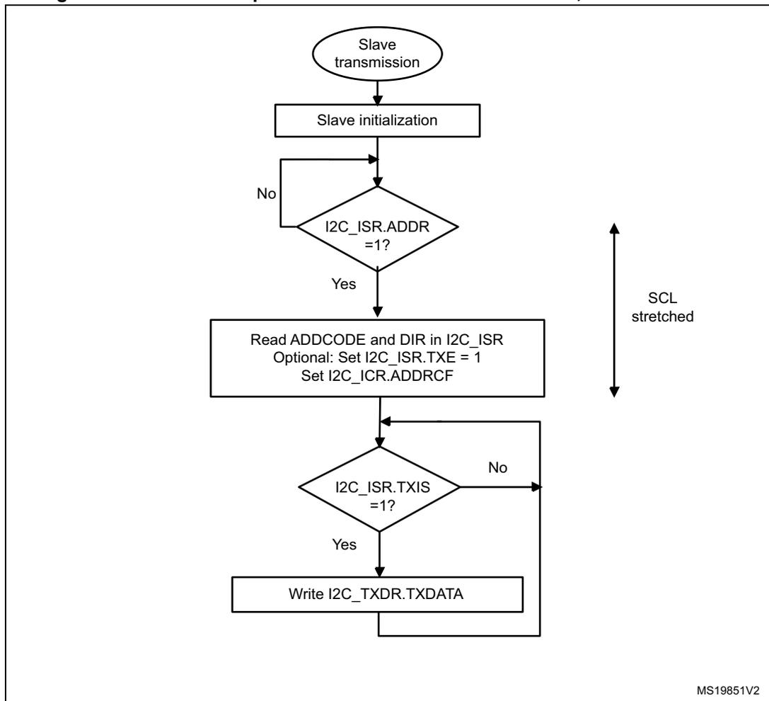
Figure 226. Transfer sequence flow for I2C slave transmitter, NOSTRETCH = 1
