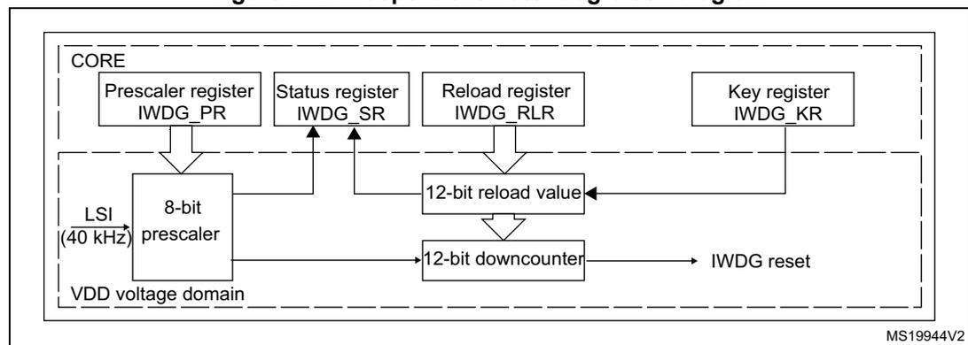
1. The register interface is located in the CORE voltage domain. The watchdog function is located in the  $V_{DD}$  voltage domain, still functional in Stop and Standby modes.
