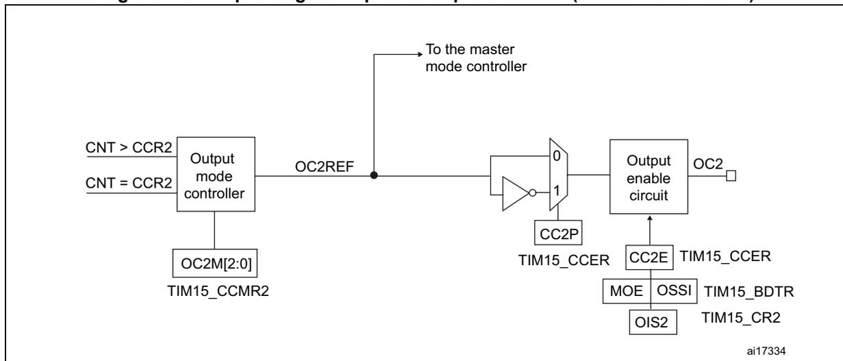
The capture/compare block is made of one preload register and one shadow register. Write and read always access the preload register.
