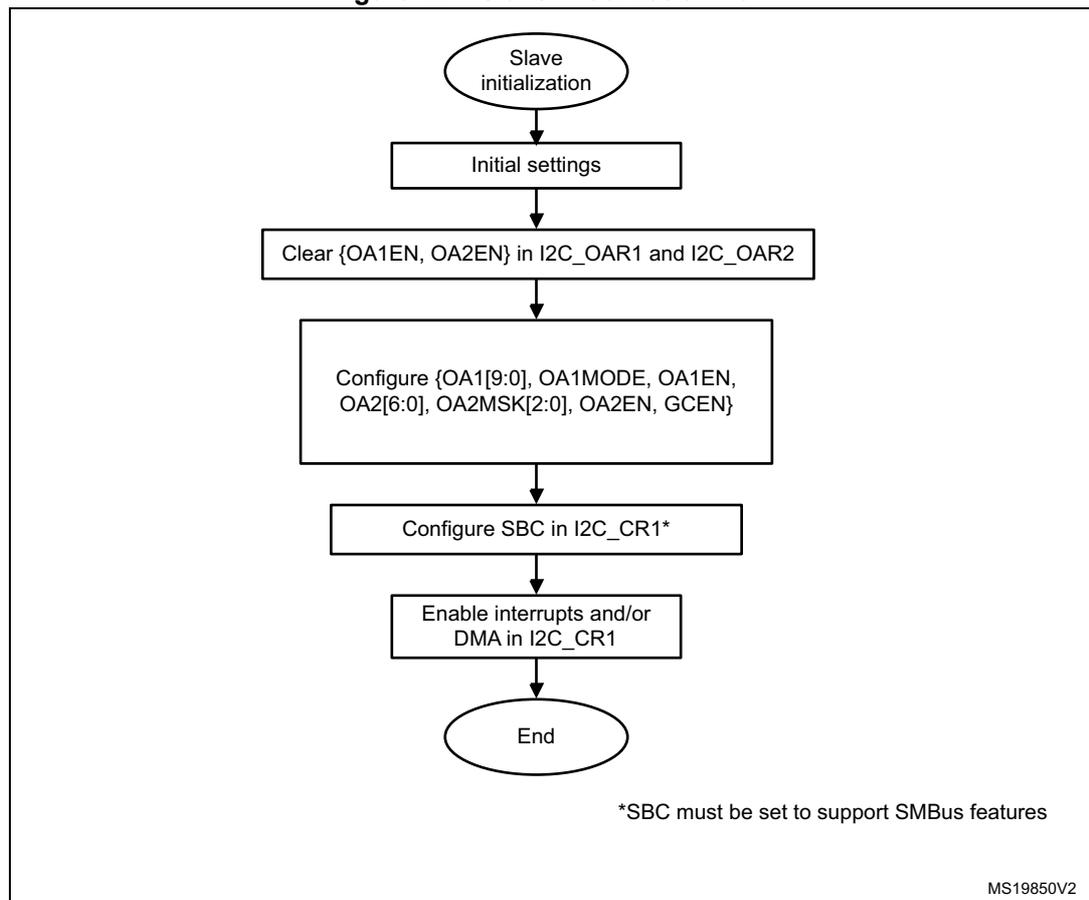
For a code example refer to [A.14.3: I2C configured in slave mode code example](#).
