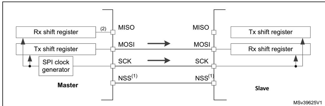
1. The NSS pins can be used to provide a hardware control flow between master and slave. Optionally, the pins can be left unused by the peripheral. Then the flow has to be handled internally for both master and slave. For more details see [Section 28.5.5: Slave select \(NSS\) pin management](#).
