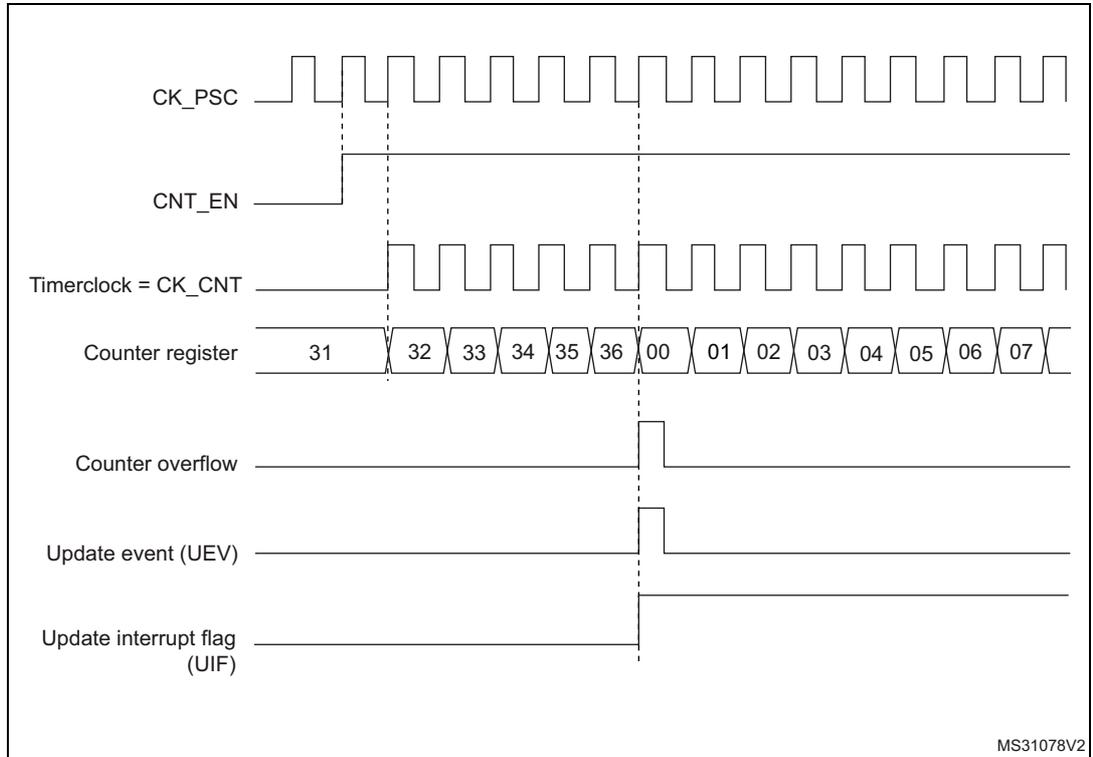
**Figure 177. Counter timing diagram, internal clock divided by 2**
