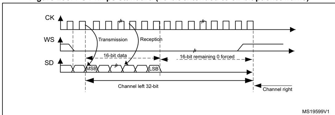
When 16-bit data frame extended to 32-bit channel frame is selected during the I2S configuration phase, only one access to the SPIx\_DR register is required. The 16 remaining bits are forced by hardware to 0x0000 to extend the data to 32-bit format.
