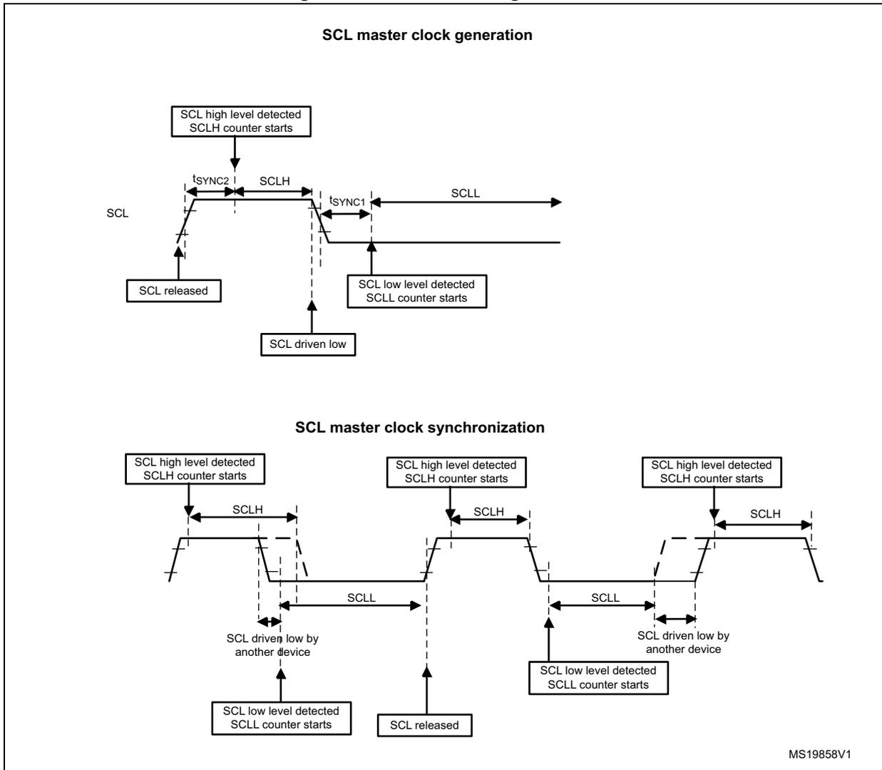
**Caution:** To be I<sup>2</sup>C or SMBus compliant, the master clock must respect the timings given in the table below.
