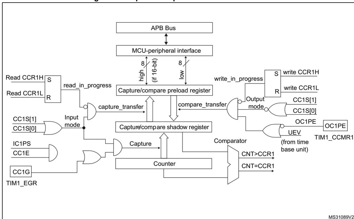
Figure 91. Output stage of capture/compare channel (channel 1 to 3)
