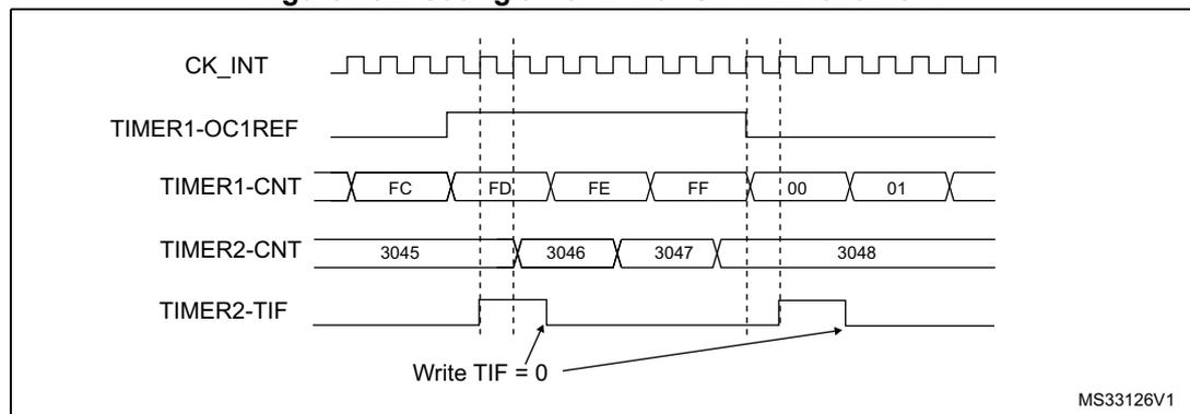
In the example in [Figure 152](#), the Timer 2 counter and prescaler are not initialized before being started. So they start counting from their current value. It is possible to start from a given value by resetting both timers before starting Timer 1. Then any value can be written in the timer counters. The timers can easily be reset by software using the UG bit in the TIMx\_EGR registers.
