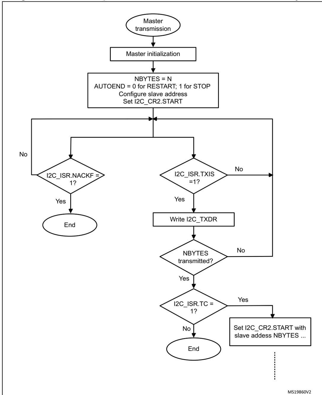
Figure 236. Transfer sequence flow for I2C master transmitter for N > 255 bytes
