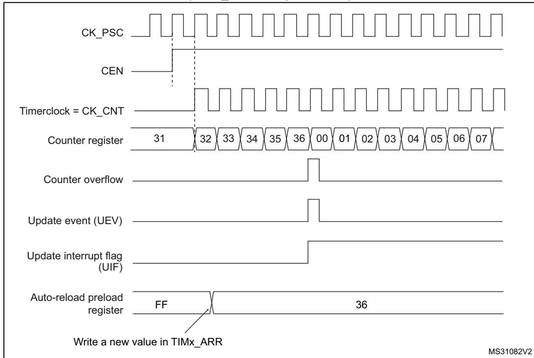
**Figure 71. Counter timing diagram, update event when ARPE=1 (TIMx\_ARR preloaded)**
