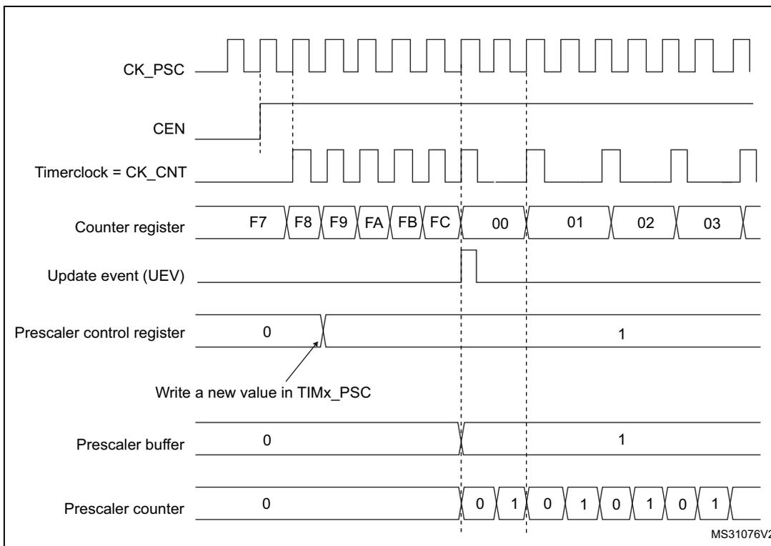
Figure 113. Counter timing diagram with prescaler division change from 1 to 4
