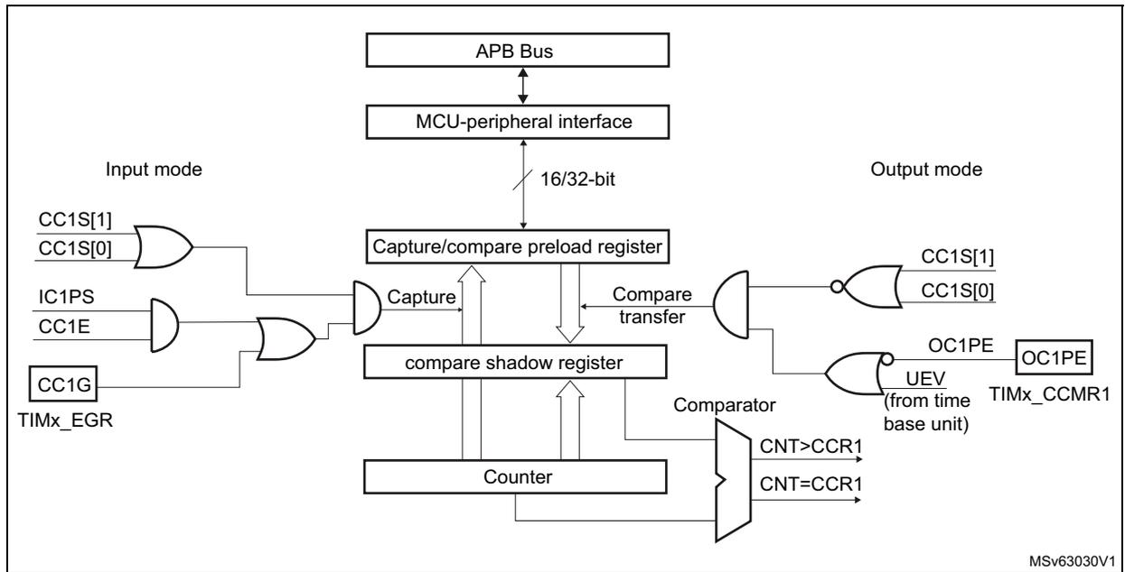
Figure 169. Output stage of capture/compare channel (channel 1)
