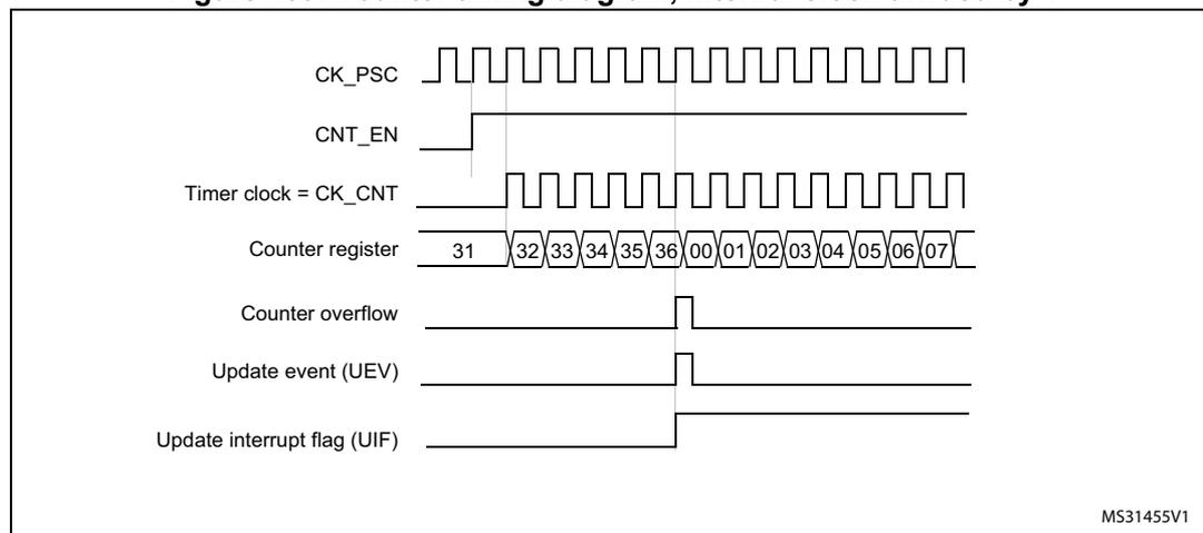
**Figure 161. Counter timing diagram, internal clock divided by 2**
