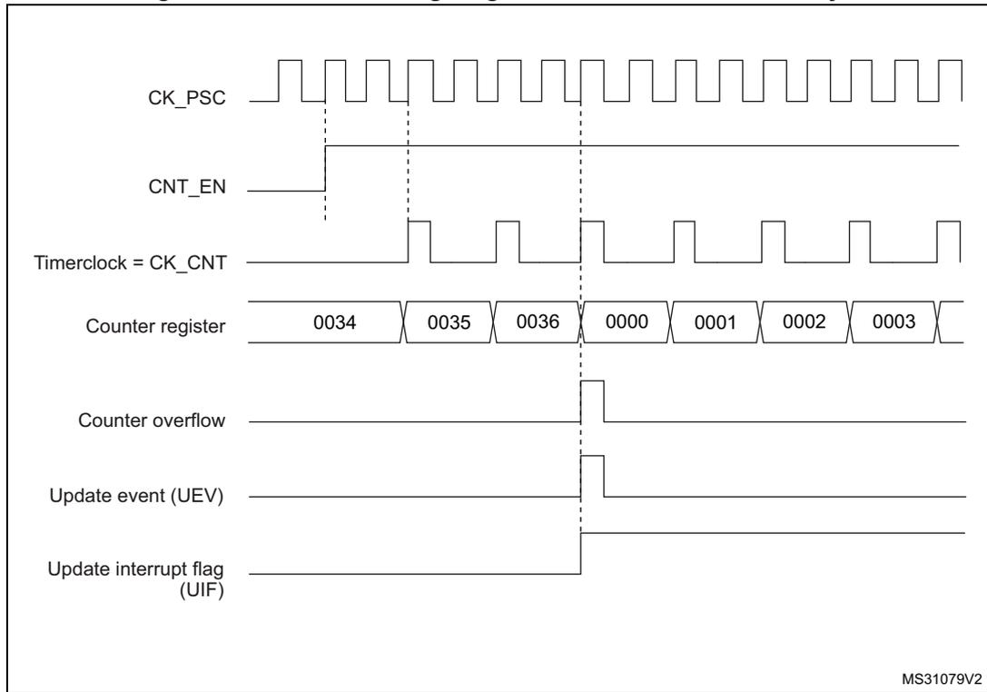
**Figure 178. Counter timing diagram, internal clock divided by 4**
