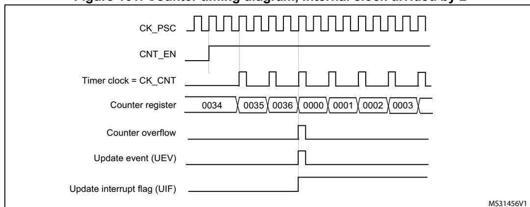
**Figure 162. Counter timing diagram, internal clock divided by 4**
