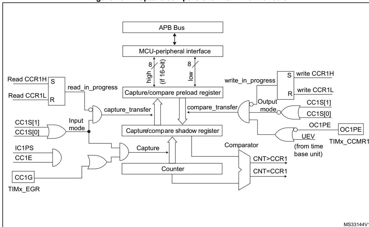
Figure 138. Output stage of capture/compare channel (channel 1)
