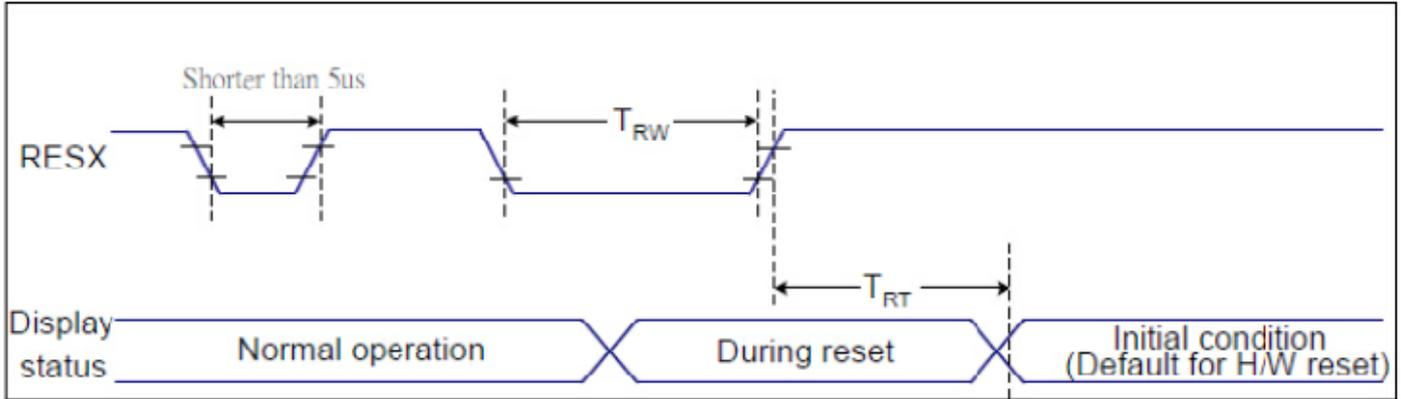
Figure 6.5: Reset Timing
