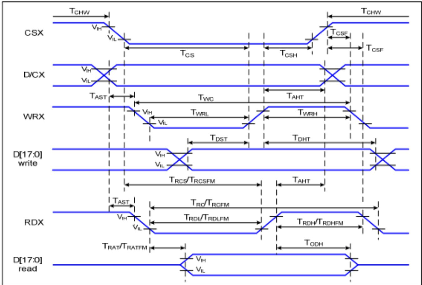
Figure 6.2: Parallel Interface Timing Characteristics (8080-Series MCU Interface)
