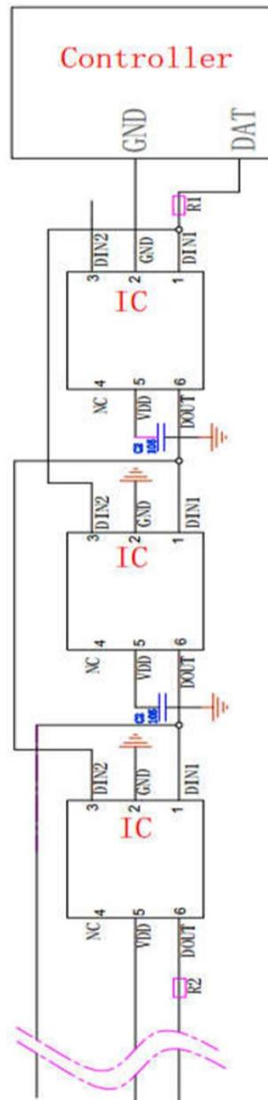
Product signal input and output must be connected in series with protection resistor R1. R1 depends on the size of the cascade amount, the greater the number of cascades, the smaller R1. The general recommended value is between 200-2K $\Omega$ , usually the recommended value is typical 500 $\Omega$ .
