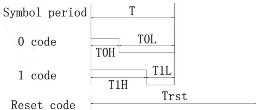
2. The data transmission time ( $T_H+T_L=1.25\mu s\pm 600ns$ ):
